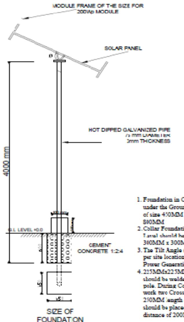
1. Foundation in Cement Concrete under the Ground Level should be of size 450MM x 450MM x 800MM
